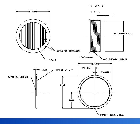
The air grill is designed to provide air distribution for crew areas, galleys, and lavatories. The air grill has light weight aluminum construction and installs with a mounting nut. PC7067-1 plenum cap assembly is available as a hose interface accessory.
