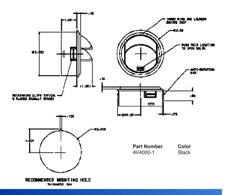
AV4000 is a two vane louver air valve made from injection molded nylon. The large orifice design of the AV4000 provides a wide air flow pattern. The vane housing rotates 360 degrees for directional control of the air stream. The anti-rotation rib on the side of the housing prevents the air valve from rotating when adjusting the vanes.
