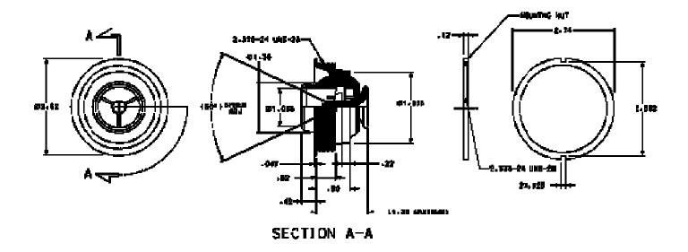
The AV4031 poppet type air valve is designed to provide high air flow volumes at low duct pressures and has minimal leakage in the closed position. The recessed ball reduces cabin protrusion which makes the air valve well suited for passenger cabin and crew area installations. The nozzle is provided in black plastic to reduce condensation and weight.
