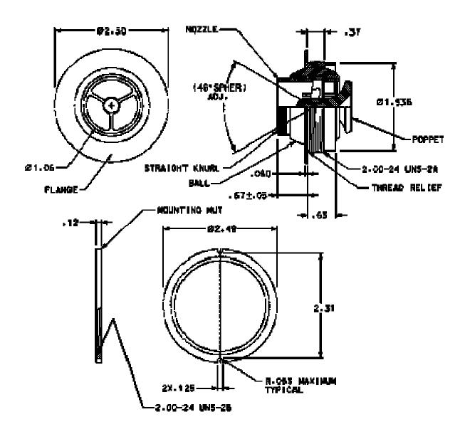
The AV4081 poppet type air valve is designed to provide high air flow volumes at low duct pressures and has minimal leakage in the closed position. The nozzle and ball are provided in black polycarbonate to reduce condensation and weight. The light weight low cost solution is well suited for single engine and light sport aircraft.
