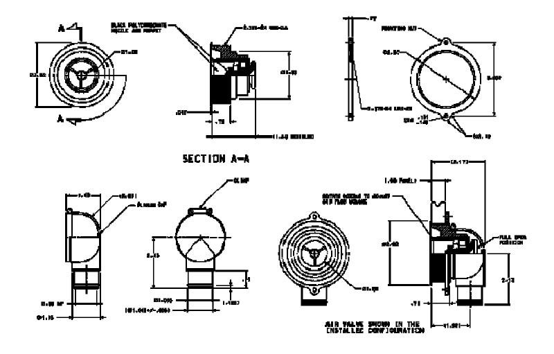
The AV4086 poppet type air valve is designed to provide high air flow volumes at low duct pressures and has minimal leakage in the closed position. The air valve is a fixed position type designed for galley cabinets and crew area installations. The nozzle is provided in black plastic to reduce condensation and weight. The air valve includes mounting nut and a plenum cap which accomdates 1.00 inch inside diameter supply hoses.
