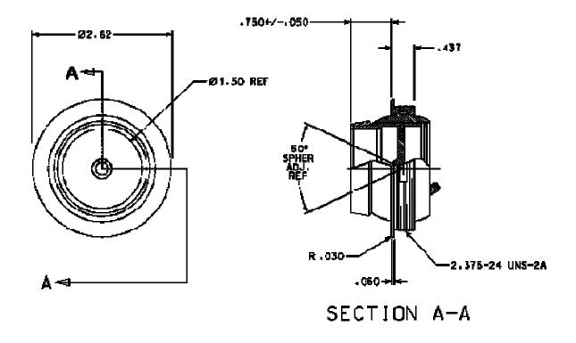
This disc type air valve is designed for high flow volumes at low duct pressure. The air valve is designed for cockpit and main cabin passenger cooling applications. Other applications are crew areas and galleys. The air valve installs with a mounting nut which is available as an accessory.
