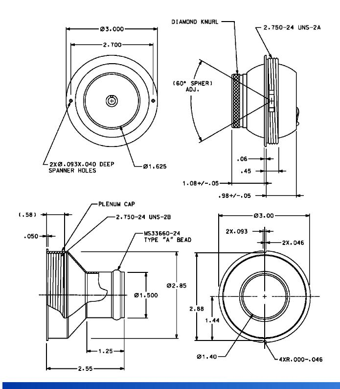
The disc type design, supplied with a clear or black anodized finish, allows for a larger air flow pattern and low air leakage. The air valve has a threaded plenum cap for ease of installation. The air valve is designed for single engine aircraft and rotorcraft.
