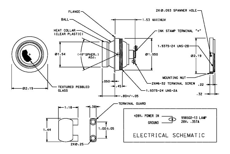
The RL6810 halogen reading light is designed for main cabin areas on general aviation aircraft. A long life Welch Allyn® halogen lamp is used in the assembly which provides a warm color spot that enhances interior surrounding. The reading light is provided with screw terminals for interface to the aircraft wiring systems and an elastomer terminal guard for terminal protection. A mounting nut is also provided for installation.
