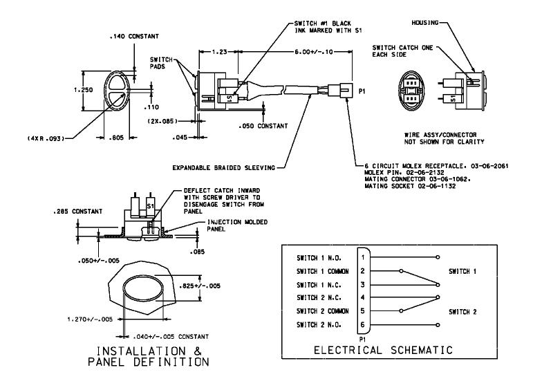
This small switch assembly is designed to switch power to a reading light and adjacent table light. Typical applications are overhead reading light and air valve panels. The switch assembly is secured by installing retainer part number 12521-1 which is available as an accessory.
