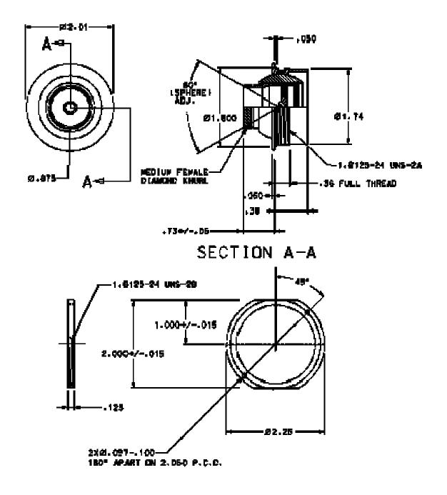
This disc type air valve is designed for high flow volumes at low duct pressure. The AV151102 maximizes air flow control and is perfect for air flow and directional control in single engine and crew areas on aircraft.
