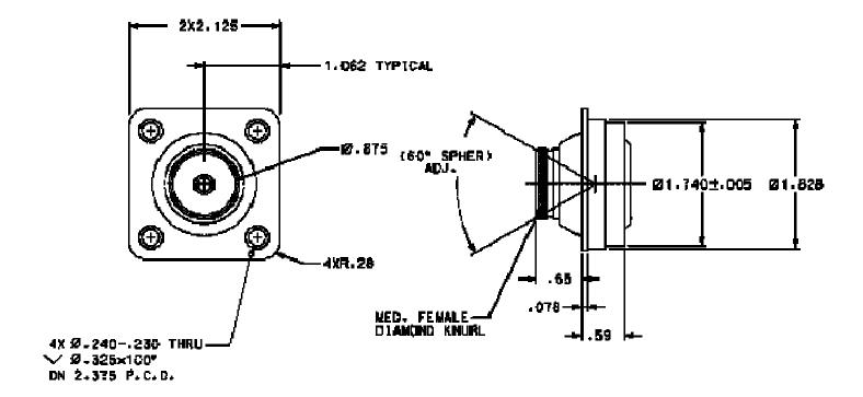
This disc type air valve is designed for high flow volumes at low duct pressure. The AV154801 maximizes air flow control and is perfect for air flow and directional control in single engine and crew areas on aircraft.
