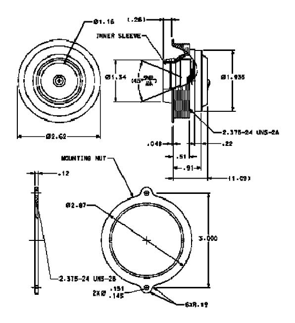
The disc type design, supplied with a clear anodized finish bright buffed to look similar to chrome, allows for a larger air flow pattern and has minimal leakage in the closed position. The recessed ball reduces cabin protrusion which makes the air valve well suited for passenger cabin and crew area installations.
