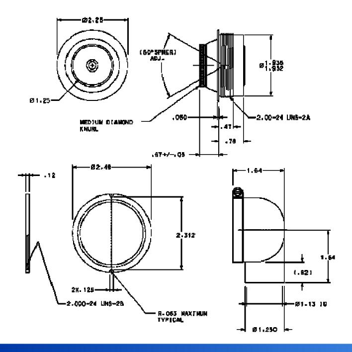
The disc type design, supplied with black or clear anodized finish, allows for a large air flow pattern and has minimal leakage in the closed position. The air valve includes a light weight plastic mounting nut and a plenum cap with 1.25 inch hose port oriented at 90 degrees.
