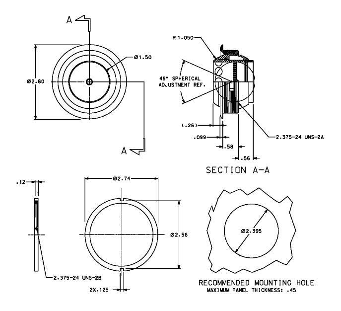
This disc type air valve is designed for high flow volumes at low duct pressure. The air valve has minimal cabin protrusion and is designed for main cabin passenger or crew areas and galleys.
