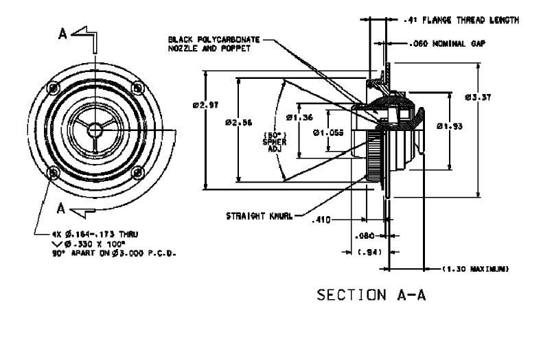
The AV4068 poppet type air valve is designed to provide high air flow volumes at low duct pressures and has minimal leakage in the closed position. The air valve is well suited for cockpit and crew area installations. The nozzle is provided in black plastic to reduce condensation and weight. The air valve is installed with four screws and has a cosmetic closeout ring for securing the adjacent panel.
