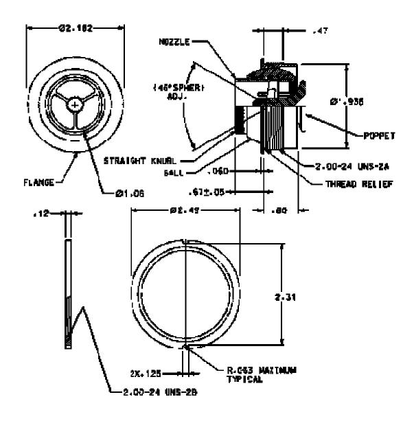
The AV4080 poppet type air valve is designed to provide high air flow volumes at low duct pressures and has minimal leakage in the closed position. The nozzle and ball are provided in black polycarbonate to reduce condensation and weight. The light weight low cost solution is well suited for single engine and light sport aircraft.
