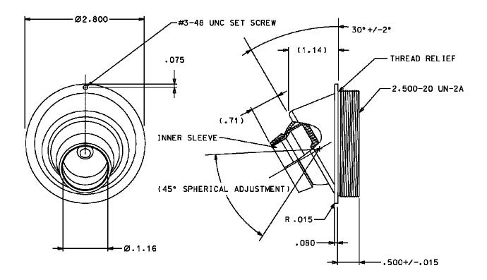
The disc type design, supplied with a clear anodized finish, allows for a larger air flow pattern and little air leakage. The angled flange on the AV4120 maximizes air flow control and is perfect for providing air along window edges and in the cockpit.
