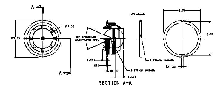
This disc type air valve is designed for high flow volumes at low duct pressure. The air valve has minimal cabin protrusion and is designed for main cabin passenger cooling applications. Other applications are crew areas and galleys.
