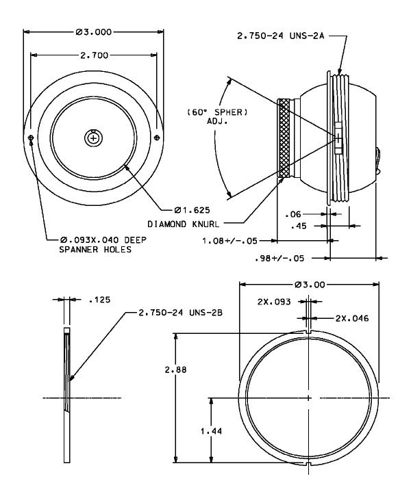
The disc type design, supplied with a clear or black anodized finish, allows for a larger air flow pattern and low air leakage. The air valve has a threaded mounting nut for ease of installation. The air valve is designed for single engine aircraft and rotorcraft.
