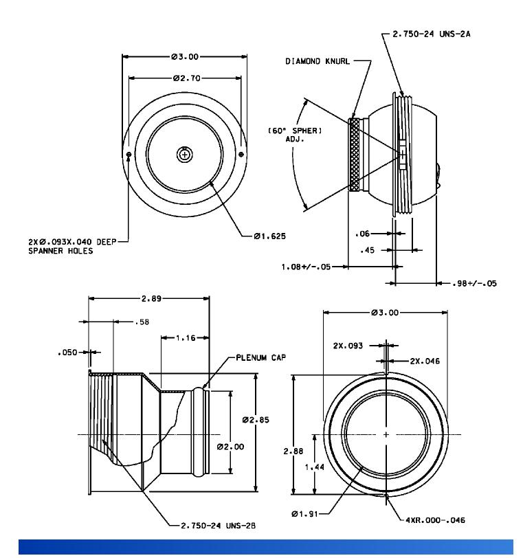
The disc type design, supplied with a clear or black anodized finish, allows for a larger air flow pattern and low air leakage. The air valve has a threaded plenum cap for ease of installation. The air valve is designed for single engine aircraft and rotorcraft.
