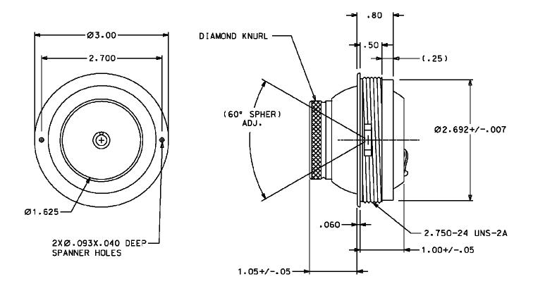
The disc type design, supplied with a clear or black anodized finish, allows for a larger air flow pattern and low air leakage. The air valve has a threaded housing for ease of installation. The air valve is designed for single engine aircraft and rotorcraft.
