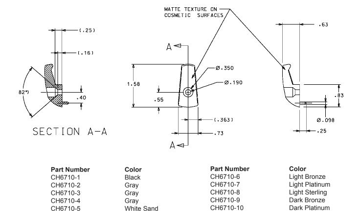
CH6710 is an injection molded plastic coat hook with a fine matte finish. The coat hook comes in an assortment of colors making it ideal for any color scheme. An anti-rotation boss on the backside of the coat hook enables it to be installed using only one screw.
