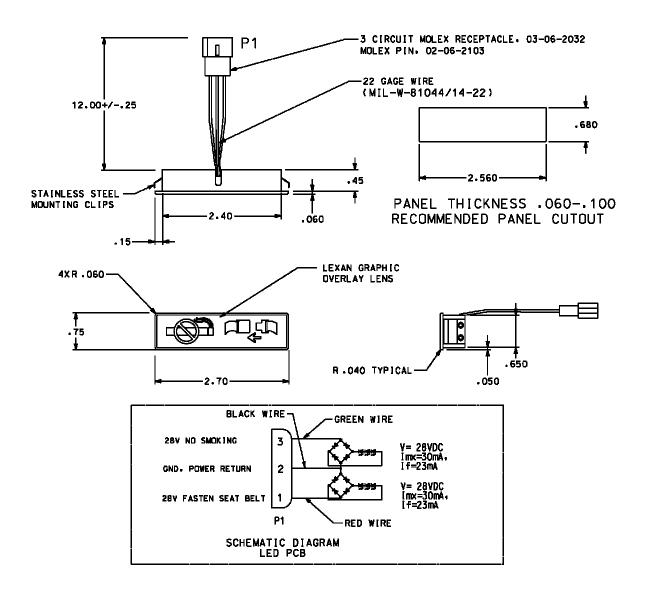
The IS5130 LED type information is a narrow low profile design with injection molded plastic bezel and utilizes long life and high quality Nichia® LEDs to provide superior operating performance for aircraft applications. The information sign is available in two standard colors of black and cream. Additional custom colors can be provided. Stainless steel mounting clips are utilized for installation of the area light in a wide range of panel thicknesses.
